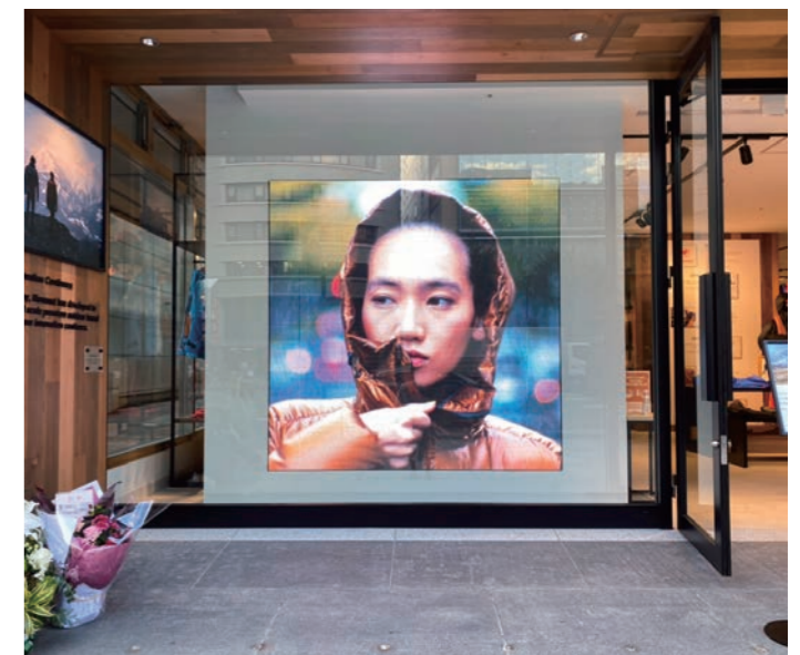
CYBER VISION: [屋外用]P3.91mm W2,000×H2,000(mm)
